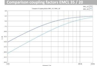
The high coupling factor of the EMCL-35 allows a test according to level 3 (10V) of IEC 61000-4-6 already at 10 kHz with the test generator CDG 6000-75\_10 or amplifier PA1020-75-250.
