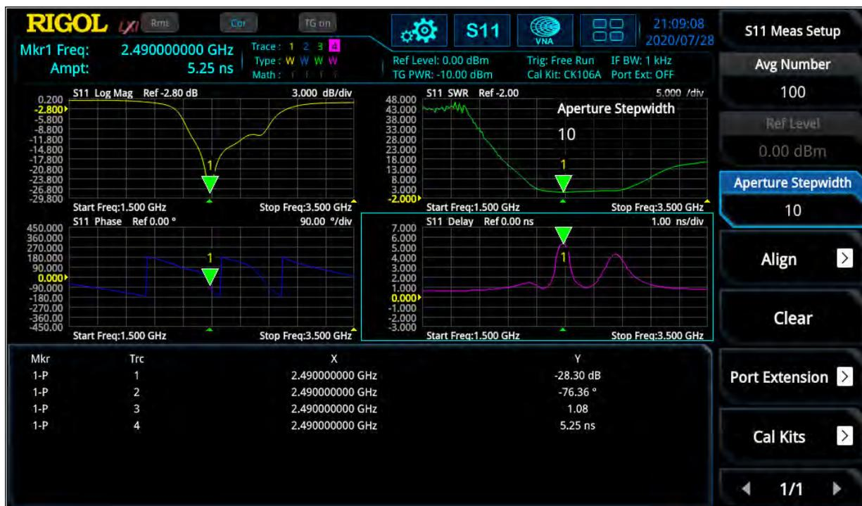
Figure 7: S<sub>11</sub> measurement: logarithmic magnitude of |r|; phase over-, SWR over- and group delay over frequency
