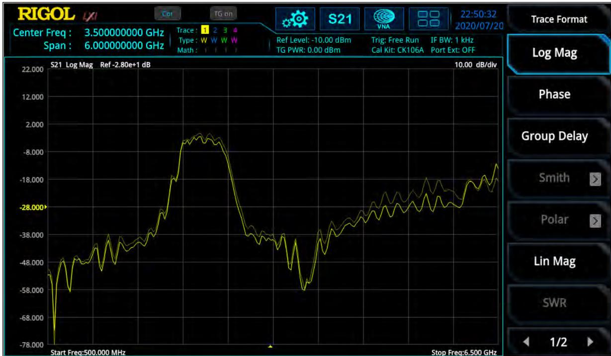
Figure 13: S<sub>21</sub> measurement of a band pass filter: Before (thin trace) and after (thick trace) Through calibration
