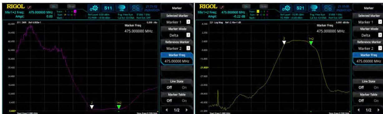
Figure 8: left side: S<sub>11</sub> SWR measurement; right side: S<sub>21</sub> insertion loss (logarithmic magnitude) measurement
