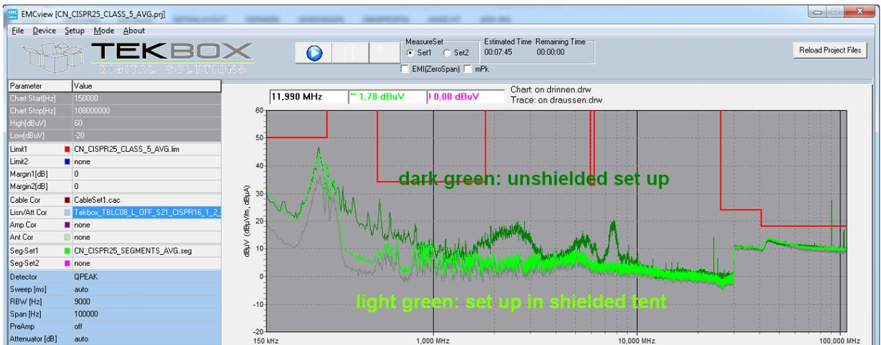
Picture 6: CISPR 25 conducted noise measurement; DUT powered
