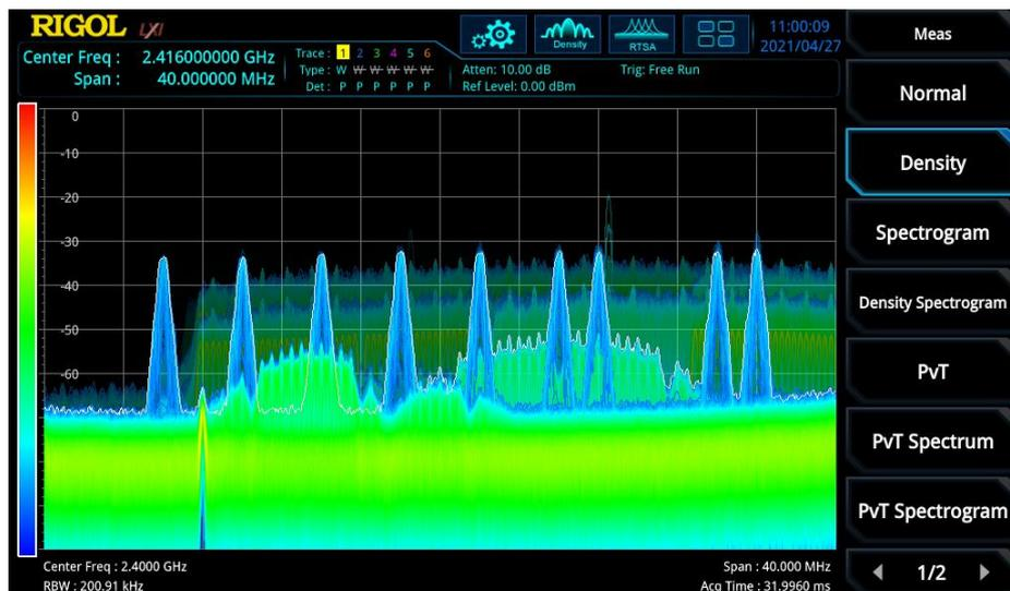
Fig. 4 Resolve co-frequency signals in the density view
