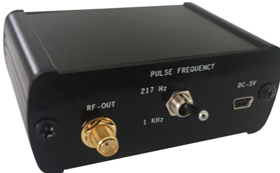
Picture 2 – TBMDA2 modulated wideband driver amplifier, rear view
