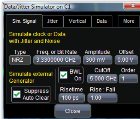
SI Studio utilizes a versatile built-in simulator as a signal source
